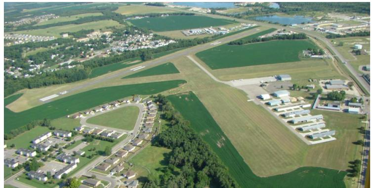
**TURF 13/31, 1915' x 150' & 5/23, 1927' x 150' Asphalt 18/36, 3495' x 75'**
